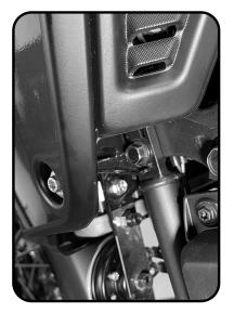
3. Attach the crash bar using the 8mm x 13mm spacer and the 8mm x 45mm bolt. Install the spacer between the sub-frame and the crash bar mounting tab.
