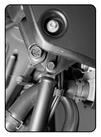
3. Attach the crash bar using the 10mm x 6mm spacer and the 8mm x 40mm bolt. Install the spacer between the sub-frame and the crash bar mounting tab.
