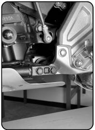
2. Remove the lower of the two bolts from the upper sub-frame bolts.
