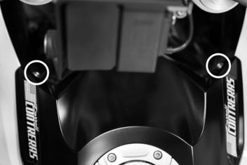
3. Remove the two T25 screws securing the small side cover. The two screws are located on the inside of the fender. Pop off the small side cover. remove the remaining 7 T25 screws securing the large side cover. Use the illustration to locate the screws. Three along the top, two on the side and the remainder inside the fender. NOTE: Keep track of the where the short and long screws go.
