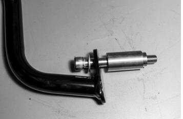
7. Remove the right side upper engine mount bolt using a T55 driver. Install the right side crash bar by using the small 13mm x 22mm x 8mm spacer. Line up the crash bar and secure it using the  $12 \times 1.75 \times 100$ mm bolt and 12mm washer. Snug down but don't tighten. Secure the front of the crash bar to the center bracket using two M8 x 1.25mm x 20 socket head cap screws.
