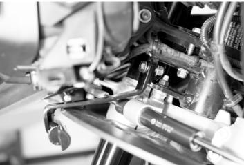
6. Remove the left side upper engine mount bolt using a T55 driver. Install the left side crash bar by inserting the large  $13 \text{mm} \times 25 \text{mm} \times 53 \text{mm}$  spacer with the narrow end first. Line up the crash bar and secure it using the  $12 \times 1.75 \times 100 \text{mm}$  bolt and 12 mm washer. Snug down but don't tighten. Secure the front of the crash bar to the center bracket using two M8 x  $1.25 \text{mm} \times 20$  socket head cap screws. Reinstall the bodywork.
