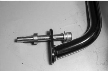
8. Tighten down the four M8 socket head cap screw securing the crash bars to the center bracket. Torque the M8 bolts to 17 ft/lb-23N/m. Torque the two engine mount bolts to 66 lb/ft (90N/m).
