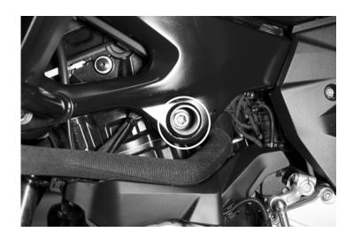
2. Install the 13mm x 22mm 46mm spacer in the engine mount bolt hole. Loosely install the crash bar using the 12mm x 80 socket head cap screw and 12mm washer. Loosely attach the lower crash bar mount to the backside of the kick stand mount using the 10mm x 25 mm bolt, washers and 10 mm Nylock nut.
