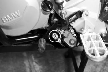
3. Remove the right side engine bolt using a T55 Torx.
