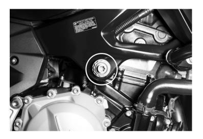
4. Loosely install the crash bar to the engine mount bolt hole using the 13mm x 22mm x 8mm spacer, 12 x 100mm socket head cap screw and 12mm washer. Loosely install the lower crash bar mount using the 10mm x 25 mm bolt, washer and the 11mm x 18mm x 10mm spacer to the side of the engine case.
