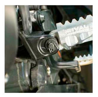
Optional step: You can adjust the brake and shifter position to better fit the repositioned pegs.
