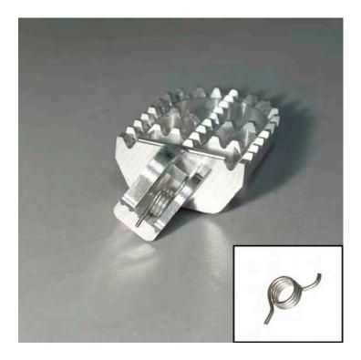
Install the peg with the straight leg in the hole on the foot peg lug.
