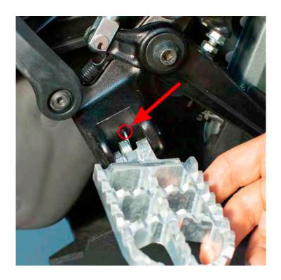
Install the factory pivot pin with the original o-ring and washer stacking the o-ring on the pivot pin first then the washer then install the cotter pin and bend the legs over to secure the pin.
