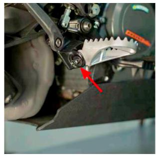
Install the factory spring in the foot peg with the straight leg facing out.
