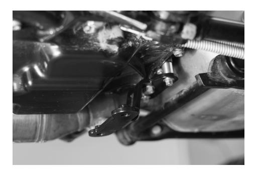
5. Attach the skid plate to the brackets using the (6) 8mm x 20mm countersunk bolts. Torque all the 8mm bolts to 17 ft/lb-23N/n.
