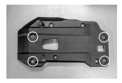
2. Remove the two factory skid plate brackets.
