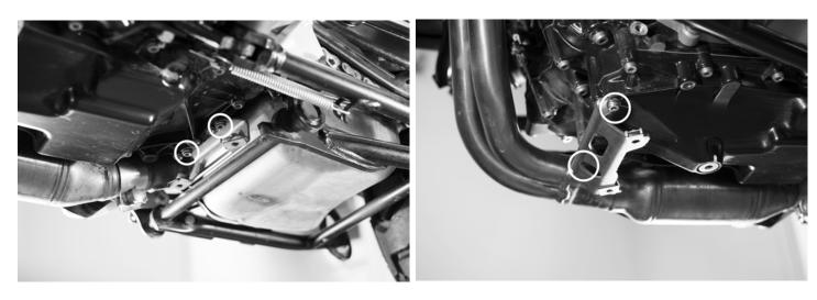
3. Loosely attach the front cross bracket to the sides of the motor using (2) 8mm x 25mm bolts and (2) 8mm washers. Attach the front lower bracket to the cross bracket using the (2) 8mm x 25mm bolts and (2) 8mm washers. Attach the bottom bracket to the motor using the (2) 8mm x 40mm bolts, (2) 8mm washers and the (2) 19mm x 17mm spacers. Torque all the 8mm bolts to 17 ft/lb-23N/n.
