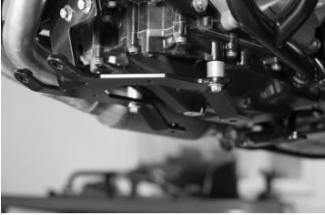
4. Install the rear bracket using the (1) 8mm x 20mm bolt, 8mm washer and the (2) 6mm x 35mm bolts, 6mm washers and the 13mm x 6mm x 15mm spacers. Torque all the 6mm bolts to 7 ft/lb-9.7N/n. Torque all the 8mm bolts to 17 ft/lb-23N/n.
