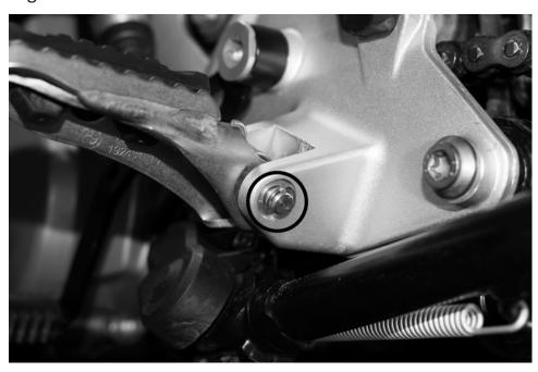
Install the supplied spring in the foot peg. Reinstall the pivot pin and secure with a circlip. Repeat on the other side.
